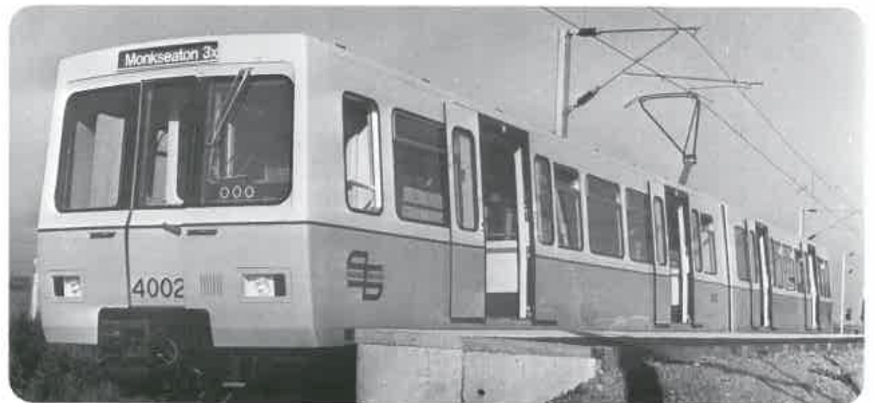
On arrival at a Metro Station the car doors can be opened by passengers pressing a button.
